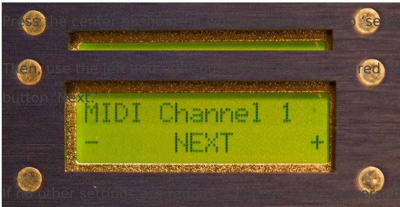
Press the center pushbutton when prompted to 'select' on the LCD screen.
