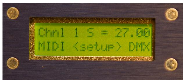
What's useful is that MIDI note messages and PC messages may be interleaved in any combination. The most recently received PC message sets the dimming speed for all subsequent note messages until a new PC message is received.
